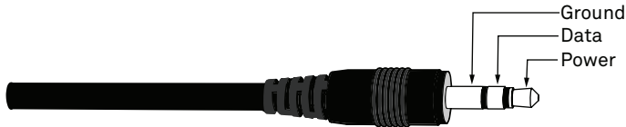
Figure 1 3.5 mm stereo plug wiring
